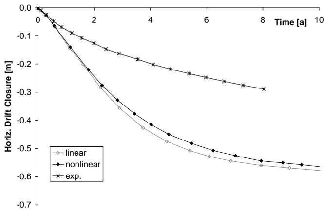
Figure 5. Calculated closure of the drift compared to experimental data.
