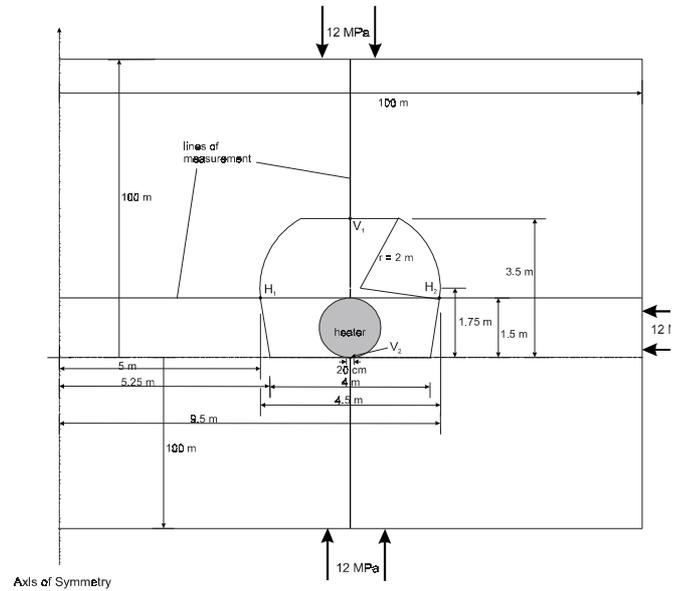
Figure 4. Sketch of the two-dimensional model of the back-filled and heated drift. The left border represents a line of symmetry.
