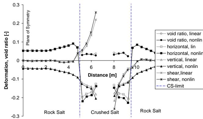
Figure 6. Deformation within crushed salt and proximal rock salt. Void ratio is also displayed.
