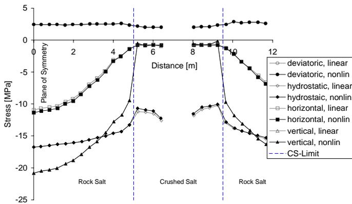
Figure 7. Stresses in the crushed salt and the proximal rock salt.
