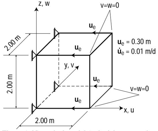
Figure 1. Numerical model (uniaxial compression test).
